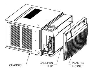
**NOTE:** Basepan clip is shipped in plastic bag with mounting screw and condensate drain cup. Install clip after reinserting chassis into outer case to prevent accidental chassis removal.
